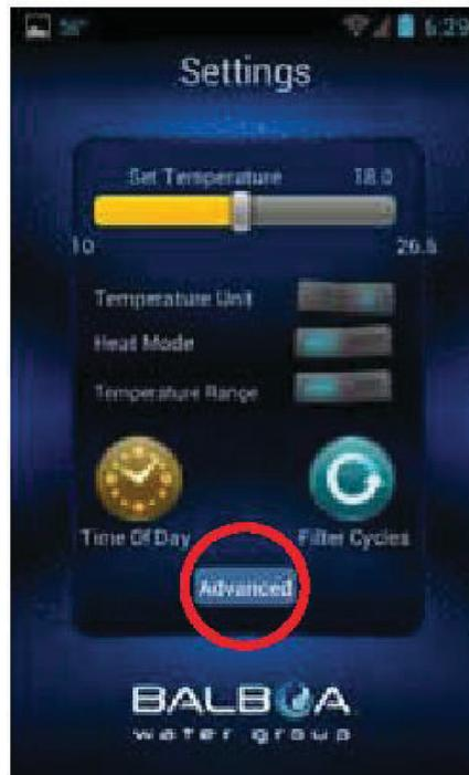
The Settings screen allows you to select the temperature of the spa, change the temperature between F° & C°, set time of day, filter cycles and more.
