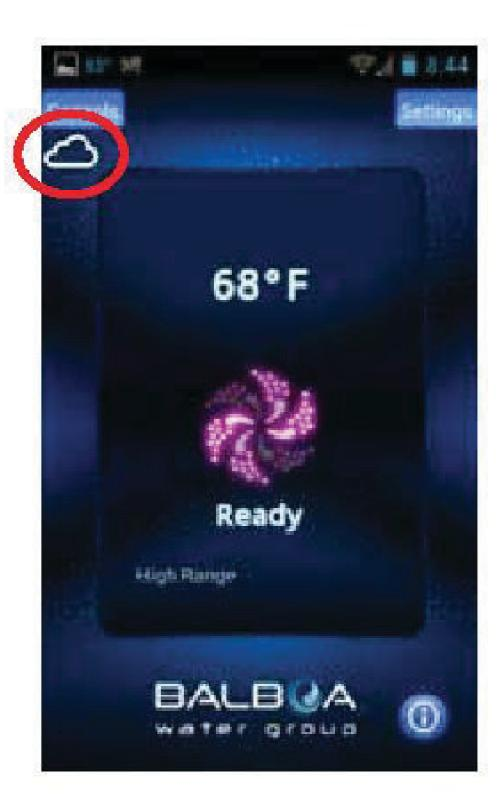
When connected via the Internet a small cloud icon will appear under the Controls button letting you know that you are remotely connected.
