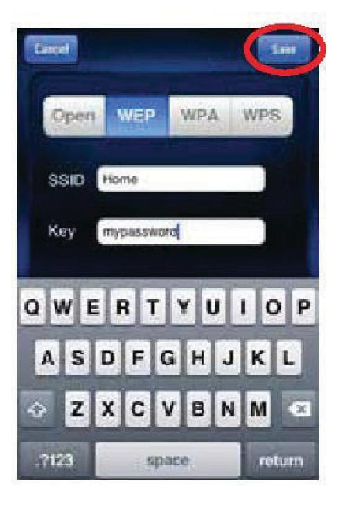
Now you will save the SSID & password to the hot tub and the tub will be ready to connect to your network.
