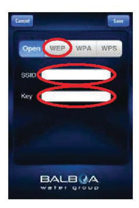
iOS setup is similar to Android except you will need to type in your SSID and Key (Password) using your keyboard.
