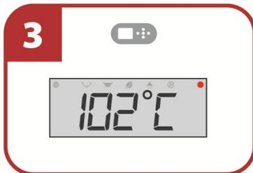
**3** Once test is complete, you will see the temperature display on your hot tub control panel.
