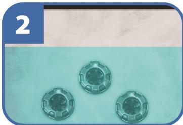
**2** When filled all massage jets should be under water (approx. 5 inches from top of spa). Remove fill hose from filter canister.
