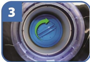
**3** Re-install filter by screwing into canister clockwise.
