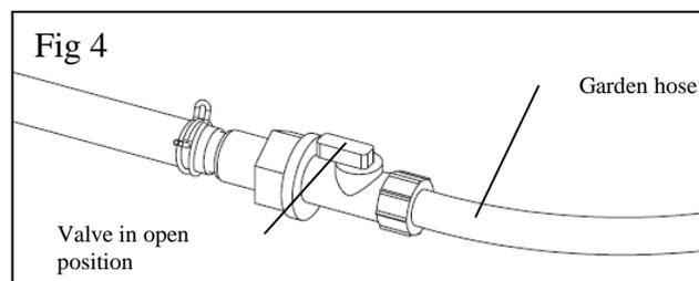
3. Route the garden hose to a sewer drain capable of safely assimilating 300 plus gallons (1135 liters) of water which may contain both unsanitary contaminants and chemical residue. Open the drain valve (as shown in Fig 4). The spa drains slowly.
