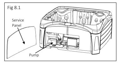
The pipes entering and leaving the pump are connected with large plastic unions. To purge the air from the pump, one of these unions will be slightly loosened.
